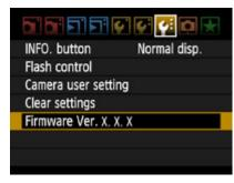
Rotate the Main Dial and the Quick Control Dial to select the "Firmware Ver.x.x.x" item at the bottom of the "Set-up 3 (Yellow)", and then press the <SET> button.
