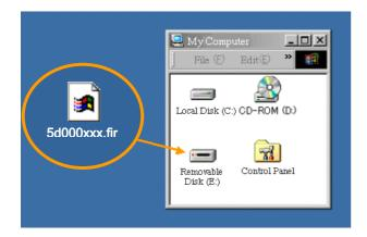
Copy the firmware update file via a card reader to a CF card that has been formatted in the Camera.
