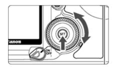
(5) Execute the firmware update after confirming the version to be installed, by selecting [OK] with Quick Control Dial and pressing the <SET> button.
