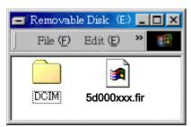
Remove the CF card from the card reader after confirming that the firmware update file has been saved to the card.
